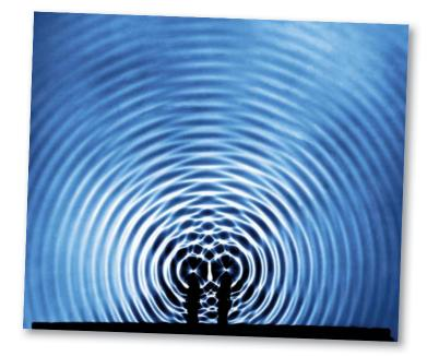
Physicists use ripple tanks to model wave motion. You know from previous work that sinusoidal functions can be used to model single wave functions. Waves are said to interfere with one another when they collide. Their collision can be modelled by the addition or subtraction of two sine waves.
