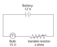
A variable resistor is used to control the brightness of a small light bulb and can be set anywhere from 0  $\Omega$  to 100  $\Omega$ . The total resistance in the circuit is the sum of the resistances of the variable resistor and the bulb.
