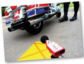
Device used to measure motorcycle noise levels
